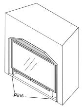
3) Bring cover plate towards the unit and hook top clip over and behind the glass frame.
